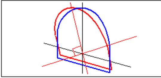
The station and offset display of points relative to a tunnel using *Point manager* or *Review job* are only calculated vertical to the alignment. If the templates were applied perpendicular in Tunnel positioning then the station and offsets will be different.
