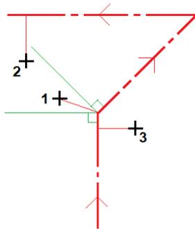
The exception to this behavior is if the distance from the point (2) to the intersection point is greater than the distance to another element in the horizontal alignment. In that case, the station and offset for the point is to the closer element.
