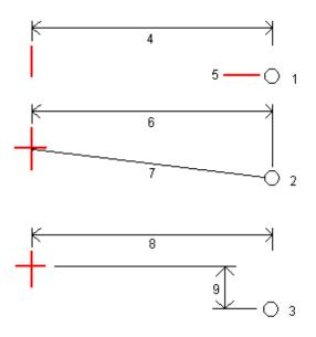
1 – **Offset and elevation**. Enter an offset (4) from the horizontal alignment, and the elevation (5) of the hinge position.
