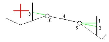
**NOTE** – For points with zero offset, you cannot apply horizontal construction offsets at the slope value of the previous line.
