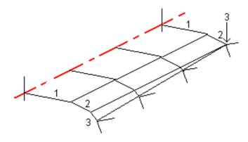
By adding strings defined with a zero offset, you can further control the interpolation process to best represent the road design.
