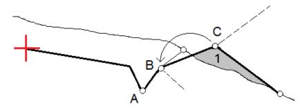
With string **B** selected as the hinge string, the cut slope can be defined by either retaining the design slope value or keying in another value. Alternatively, the cut slope can be defined by selecting one of the following:
