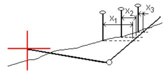
The plan view shows the calculated catch position. The calculated slope value (in blue) and the design slope value appears at the top of the screen.
