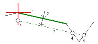
**NOTE** – You must be in the cross section view to define a subgrade. You cannot define a subgrade from the Stakeout method screen or when measuring your position relative to a road or a string.
