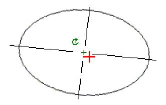
Tap and hold on a position to see its horizontal and vertical offsets, northing, easting, and elevation. If the design alignment has been offset, the reported offset values are to the offset alignment. If rotation has been applied and the pivot position has been offset, the reported offsets are to the offset position.
