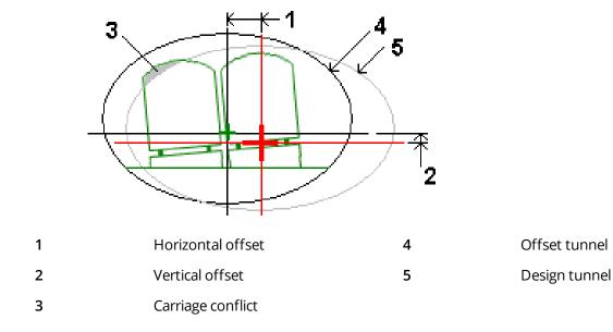
To add alignment offsets to the tunnel definition, see To add alignment offsets, page 24.
