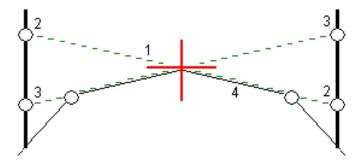
Typically a wire (1) is stretched from one side of the road to the other fixed at position (2) on each stake. The wire is then checked to see that it lies on the formed road surface (4). The process is then repeated for the other side of the road by fixing the wire to the stakes at position (3). The cross slope can be offset vertically so that the wire is above the surface making it easier to confirm the construction. If the
