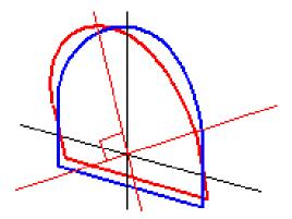
The station and offset display of points relative to a tunnel using **Point manager** or **Review job** are only calculated vertical to the alignment. If the templates were applied perpendicular in Tunnel positioning then the station and offsets will be different.
