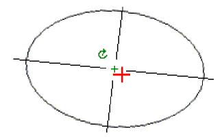
Tap and hold on a position to see its horizontal and vertical offsets, northing, easting, and elevation. If the design alignment has been offset, the reported offset values are to the offset alignment. If rotation has been applied and the pivot position has been offset, the reported offsets are to the
