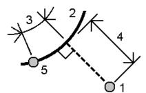
The distance along the arc (3) and the perpendicular distance (4) to the arc is calculated. The distance along the arc is from the point specified (5).
