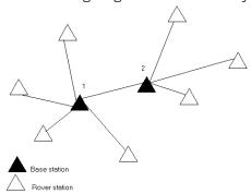
In this survey, Base station 2 was first surveyed as a roving point from Base station 1.
