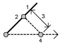
The software calculates the following values: computed azimuth (4), from the start point of the line to the offset point, and the computed angle, measured clockwise between the line and the azimuth (4).
