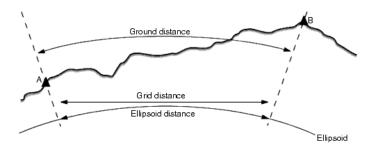
**NOTE** – If the coordinate system for a job is defined as **Scale factor only**, ellipsoid distances cannot be displayed.
