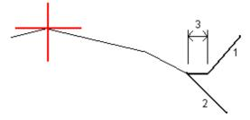
**TIP** – When staking a side slope the hinge position and, if applicable, the cut slope hinge position are displayed in the map and can be selected and staked.
