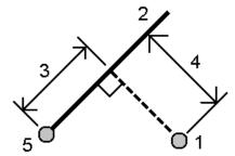
The distance along the line (3) and the perpendicular distance (4) to the line is calculated. The distance along the line is from the point specified (5).
