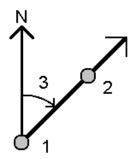
The software calculates the azimuth between the entered values (3).
