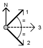
The software calculates the following values: the azimuth halfway between the entered values (3) and the computed angle, measured clockwise between azimuth 1, and azimuth 2.
