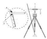
**NOTE** – Measure the height to three different underside notches around the perimeter of the groundplane. Then record the average as the uncorrected antenna height.
