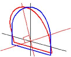
The station and offset display of points relative to a tunnel using **Point manager** or **Review job** are only calculated vertical to the alignment. If the templates were applied perpendicular in Tunnel positioning then the station and offsets will be different.
