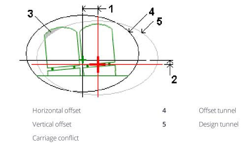
To add alignment offsets to the tunnel definition, see **To add alignment offsets, page 22**.
