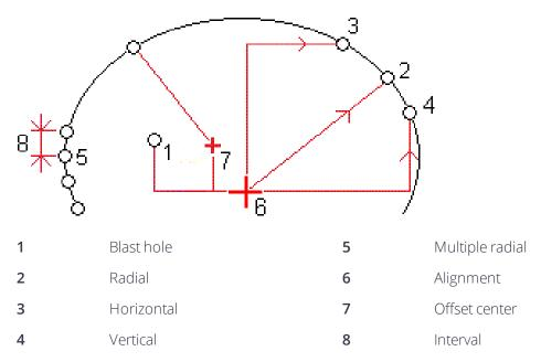
For each method, you must specify the **Start station** and **End station** and, if required, the horizontal or vertical offset and the direction of the offset. Horizontal and vertical offsets are relative to the alignment. If the alignment has been offset, the offsets are relative to the offset alignment.
