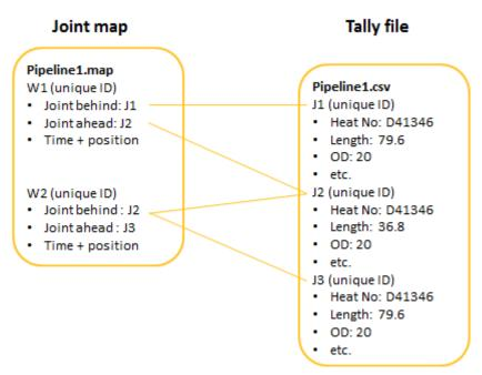
In this example, the weld W1 is linked to the joints J1 and J2. If required, the details for J1 and J2 can be updated during joint mapping and the changes are saved in the tally file.
